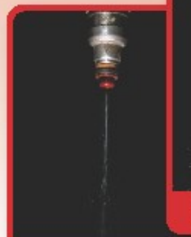
Fouled fuel injector produces irregular spray pattern.
