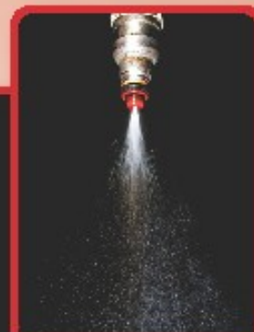
Clean fuel injector displays proper spray pattern.
